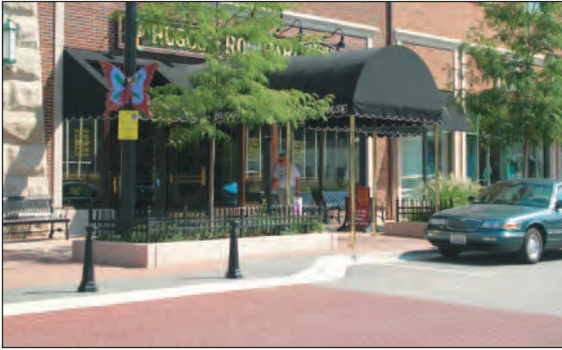
A mid-block crossing helps improve pedestrian safety and mobility by providing a clearly demarcated crosswalk located between the typical crosswalks at intersections.
